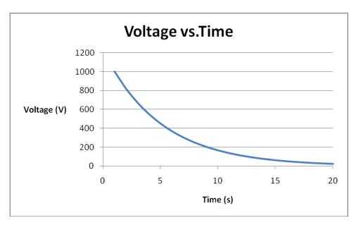
At time t = 5 seconds, the voltage is about 450 V. Therefore, the current is 45 A (anything between 40 and 50 would be accepted).
