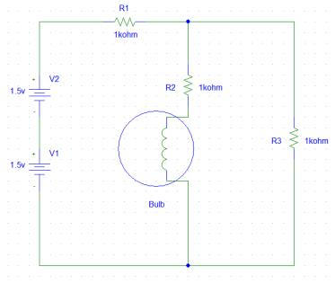
Station 3: Determine the equivalent resistance of the constructed circuit.
